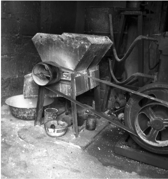
FIGURE 5. A Gari processing machine (photograph, author, 2012)
