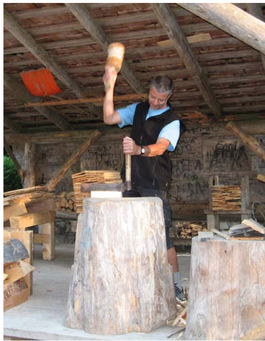
Ballenberg Open Air Museum showing the making of wooden tiles for roofing.
