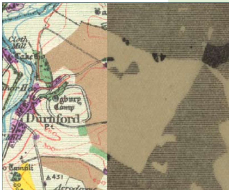
Figure 4 (below) – Comparing the green layer colour separation for part of the Salisbury and Bulford area with an adjacent area of the published LUSGB map. The solid areas on the separation are woodland and the striped areas are pasture.
